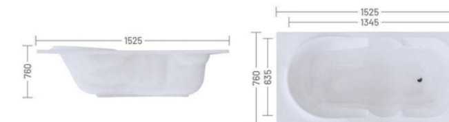
WBT-005 Length 1525mm Breadth 760mm Depth 405mm Waste Hole Distance from wall 350mm
